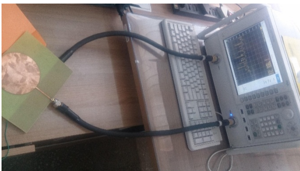
Figure 9: Antenna connected to Vector Network Analyzer
